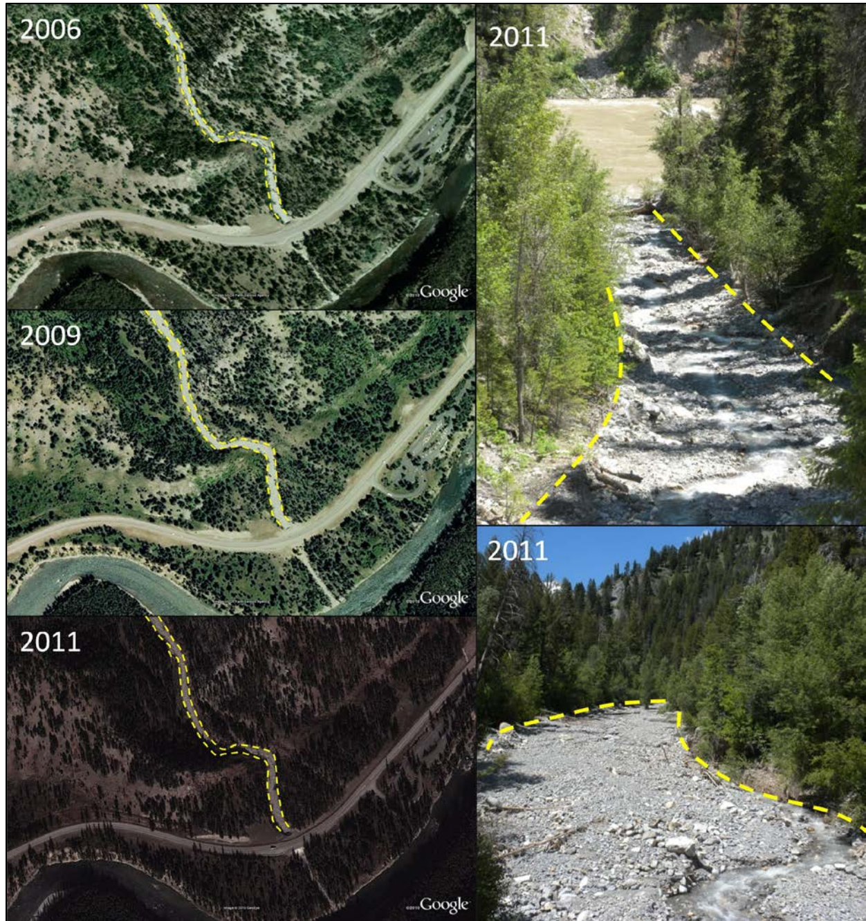
Figure 15. Remotely sensed images from 2006, 2009, and 2011 acquired from Google Earth (left) and ground-based images from 2011 (right) of a non-perennial stream in Teton County, WY. The acquired remotely sensed images allow for a preliminary off-site delineation of the OHWM (indicated by a dashed line). Visual analysis of this time series of remotely sensed images suggests relatively stable active channel boundaries from 2006 to 2011. Field validation of the off-site delineation verifies that the active channel signature identified in the remotely sensed images corresponds with the field signature as expressed by three primary indicators—break in slope, change in sediment characteristics, and change in vegetation characteristics.
